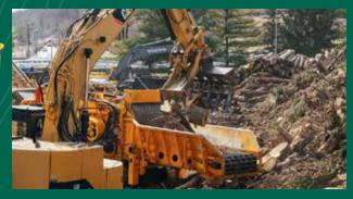
60" WIDE INFEED & ROTOR: THE 5900T SIGNIFICANTLY ENHANCES MATERIAL FLOW, EFFORTLESSLY HANDLING WIDER MATERIAL AND REDUCING THE NEED FOR PRE-PROCESSING.
